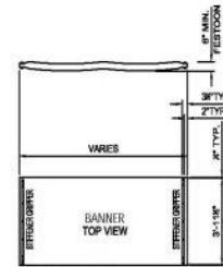
9 L-066 SCALE: NA STIFFENER/GRIPPER DETAIL NOTE: MIN. FESTOON DEPTH REQUIREMENTS ARE DEPENDENT ON THE CABLE LENGTH.
